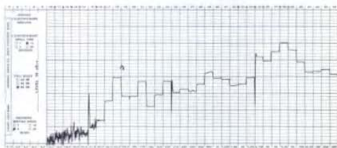
Figure 2. A stepped 1/3-octave analysis of vibration of defective motor. Dwell time was set at 10 seconds, full-scale level was 80 dB, and recorder writing speed was 3 in./s. Chart paper is GR 1521-9460, specially designed for stepped 1/3-octave analysis.
